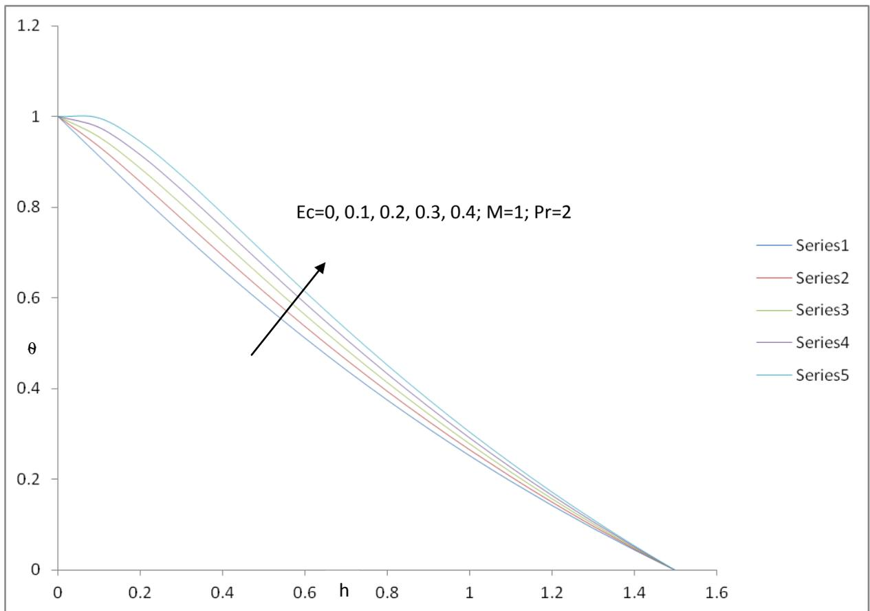
Fig 4 Temperature profile for different values of  $E_c$  for  $M=1, Pr=2$
