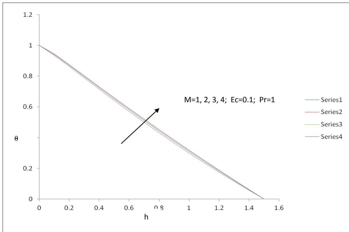
Fig 2 Temperature profile for different values of M for  $Ec=0.1, Pr=1$
