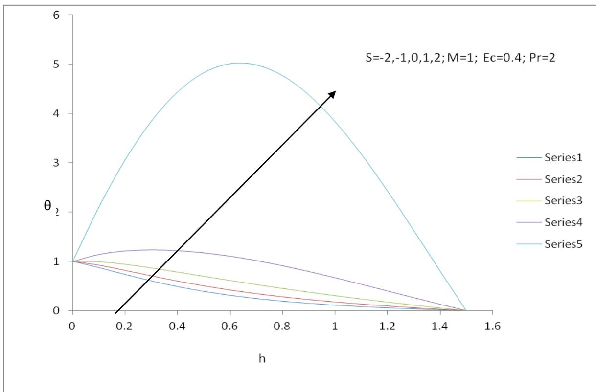
Fig 5 Temperature profile for different values of  $S$  for  $E_c=0.4, M=1, Pr=2$
