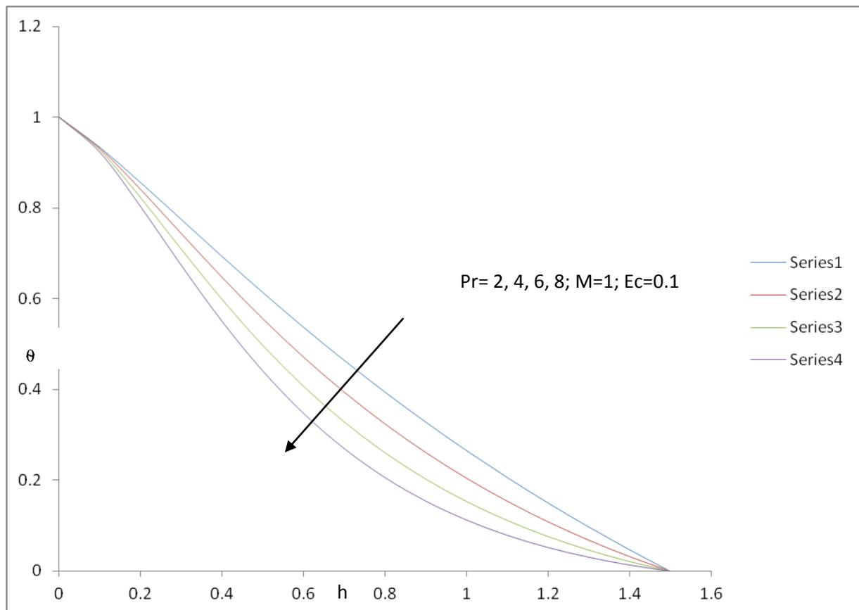
Fig 3 Temperature profile for different values of Pr for  $Ec=0.1, M=1$
