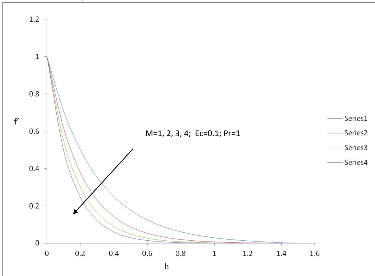
Fig1 Velocity profile for different values of M for Ec=0.1,Pr=1
